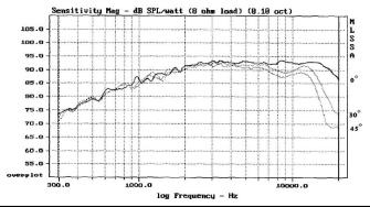
Measured on IEC baffle using Bruel & Kjaer 3144 model microphone. Also available in black faceplate finish.
